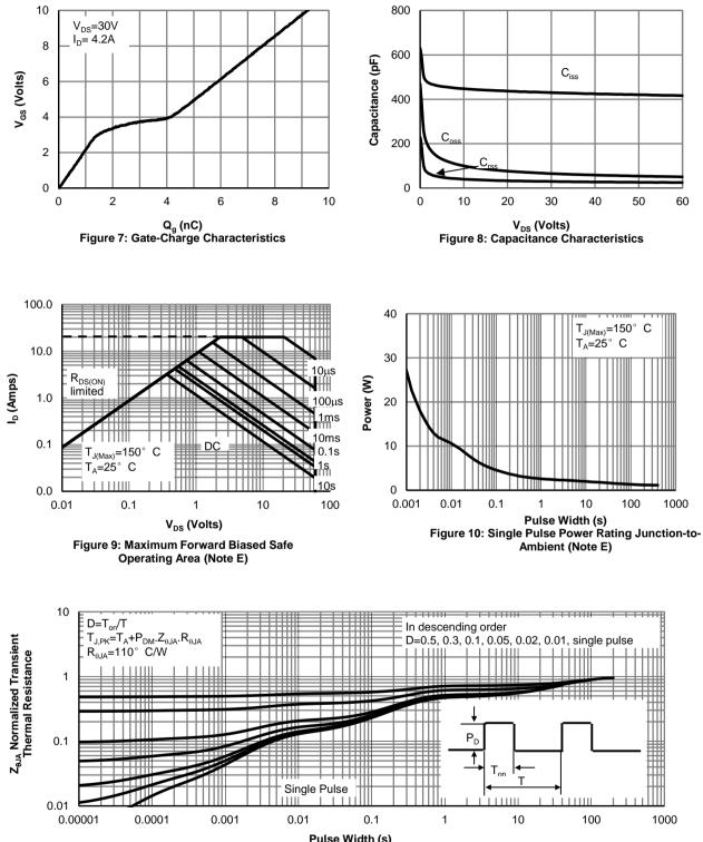
Pulse Width (s) Figure 11: Normalized Maximum Transient Thermal Impedance
